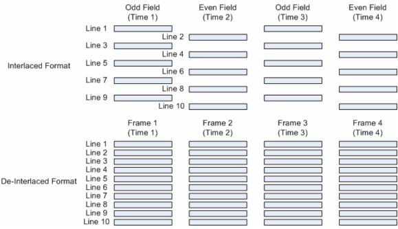
Figure 7. Interlaced Format versus De-Interlaced Format
